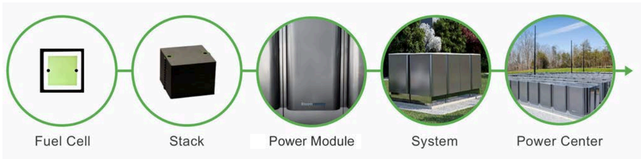
Figure 2: Energy Server Architecture
