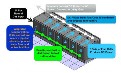
Bloom desulfurization canisters - the first processing units in the server array – are designed to remove sulfur odorants from the natural gas feedstock. The sulfur odorants, if not removed, would rapidly and irreversibly damage the fuel cells, disabling the production of electricity.
