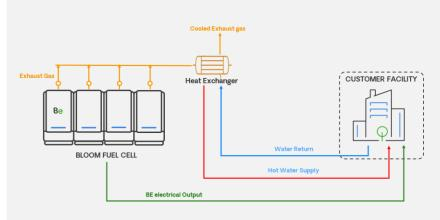
2,777 kg/hr of hot water per 325kWe of fuel cell
