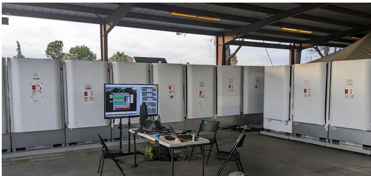
Figure 6. Bloom Testing System dedicated to simulating and supporting dynamic loads (see configuration in Figure 7)
